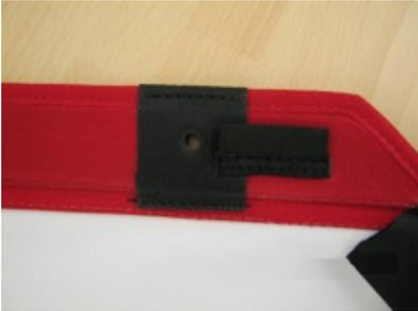
Re-attach cutter keeper according to Airtec Riggers Manual
