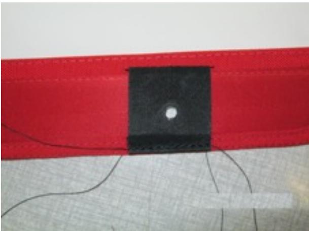
Fold under excess material and sew on
