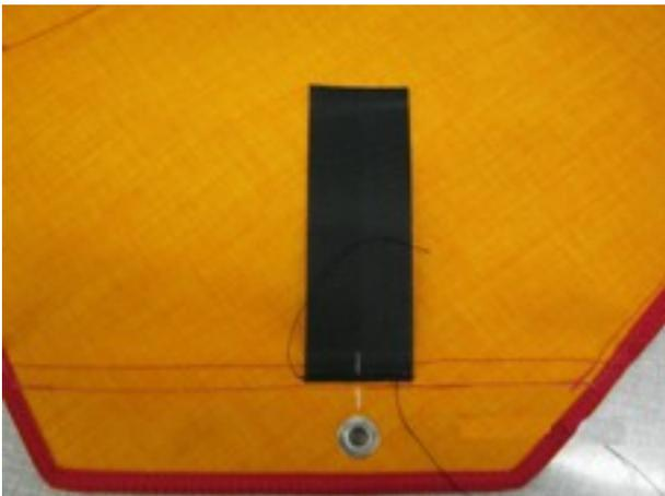
Place 12 cm Type XII piece onto outside of flap, line up with grommet centre and sew it on
